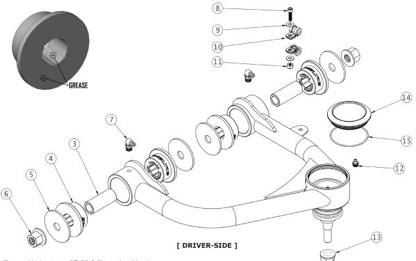
Torque M14 nuts to 85-90 ft/lbs, w/ red loctite
